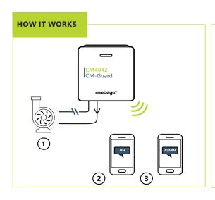
The Mobeye CM4042 monitors various fault contacts or sensors of your installation and allows remote switching of a device, pump or motor switch.
