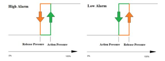
Return Stroke Error = | Action Pressure - Release Pressure |
